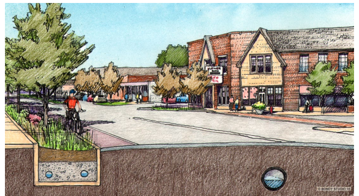
Tree planters with stormwater filtration
